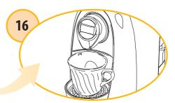
If the container fills up, empty it out and replace until the prime/rinse cycle is complete.
