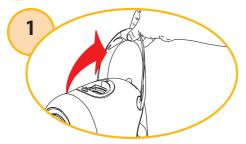
Turn machine off. Raise the lever to open the capsule compartment.
