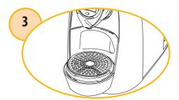
The grill must be positioned over the drip tray turned.
