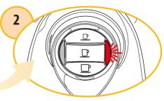
The alarm indicator light will blink and beep. The machine will immediately stop dispensing.
