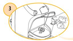
Remove and empty out the water tank.
