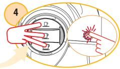
Keep the beverage buttons pressed down and simultaneously switch the machine on.
