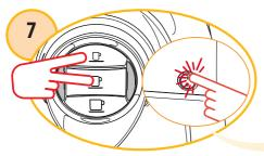
Keep the espresso and long espresso buttons pressed down and simultaneously switch the machine on.
