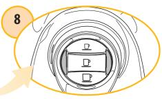
The selected beverage button will blink. The machine will stop dispensing beverage on reaching the programmed quantity, and beep.
