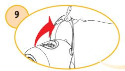
Raise lever to eject used capsule into the used capsule drawer.
