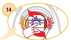
The long espresso button and the descale and alarm indicator lights blink alternately. Press the long espresso button to start the prime/rinse cycle.
