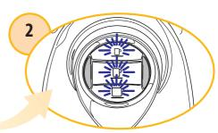
The beverage buttons will blink simultaneously to indicate that the machine is warming up. When the buttons remain steadily lit, the machine is ready for use.
