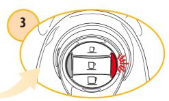
The alarm indicator light will blink and beep three times to confirm deactivation of the "Energy Saving" function. When the function is reactivated, the alarm indicator light will blink and beep two times.
