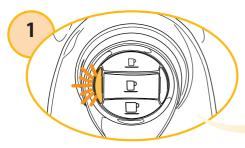
When the descale indicator light blinks and the machine beeps, it is advisable to carry out a descaling cycle.
