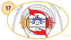
At the end of the prime/rinse cycle, the long espresso button and the descale and alarm indicator lights blink alternately and the machine beeps.
