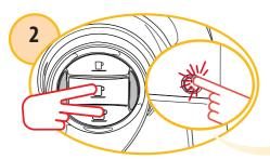
Keep long espresso and brewed coffee/tea buttons pressed down and simultaneously switch machine on.
