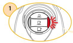
When the alarm indicator light blinks and the machine beeps, the water tank is empty.
