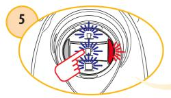
Press the long espresso button once. Wait approximately 2 minutes for the machine to complete the priming cycle. During this cycle, the alarm indicater light will blink. The alarm light will go off and the 3 beverage buttons will blink to confirm the end of the priming cycle. Repeat this step only if the alarm indicator light continues to blink.
