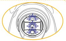
To restore normal operating conditions, press any beverage button or raise the lever. The machine will warm up. When the machine is ready for use, the beverage buttons will be steadily lit.
