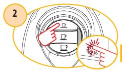
Press and hold down the espresso button while simultaneously switching the machine on.
