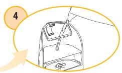
Prepare the descaling solution following the manufacturer's directions and pour a liter of solution into the tank.
