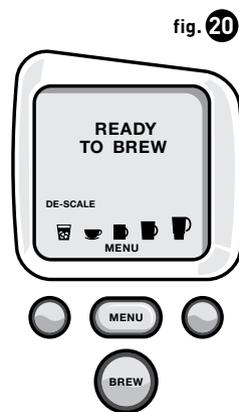
The Brewer should be de-scaled every 3-6 months to ensure optimal performance. It is possible for calcium deposits to build up faster, making it necessary to de-scale more often.
